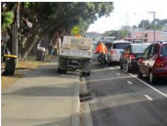
Figure 2-14: Photo showing a combination of vehicles parked across the buffer zone and on the footpath, limiting the width available to the cyclist
