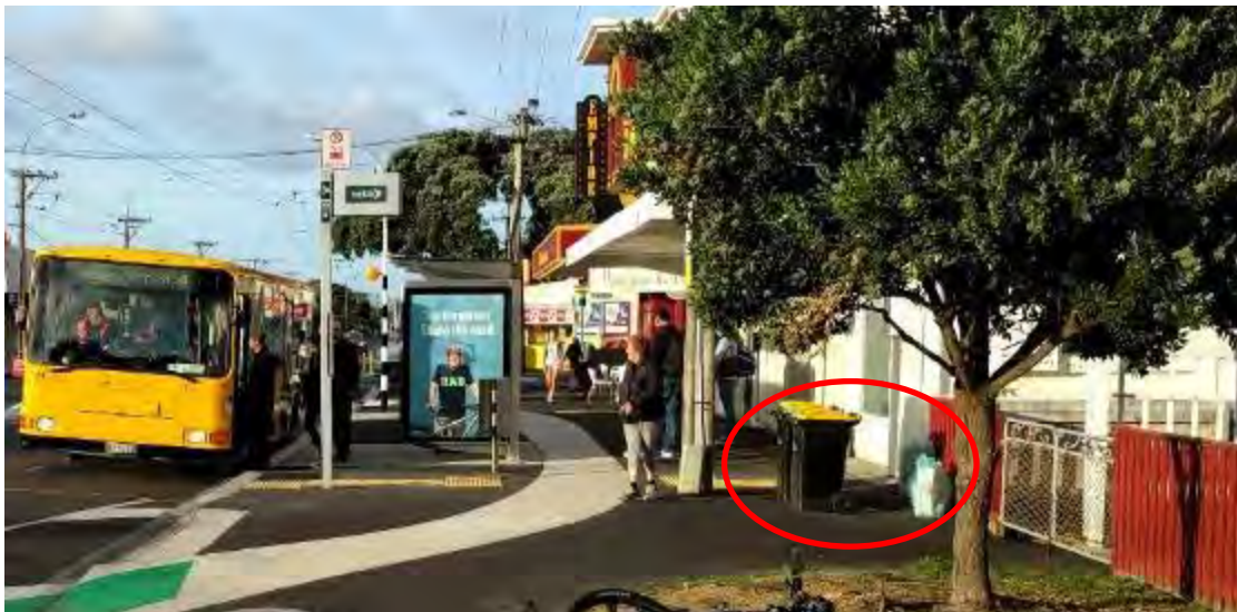
Figure 2-33: Photo showing bins obstructing the shared space at the Mersey St bus stop bypass
