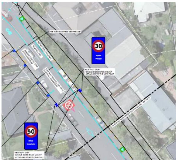
Figure 2-15: Speed limit change location along Kenya Street
