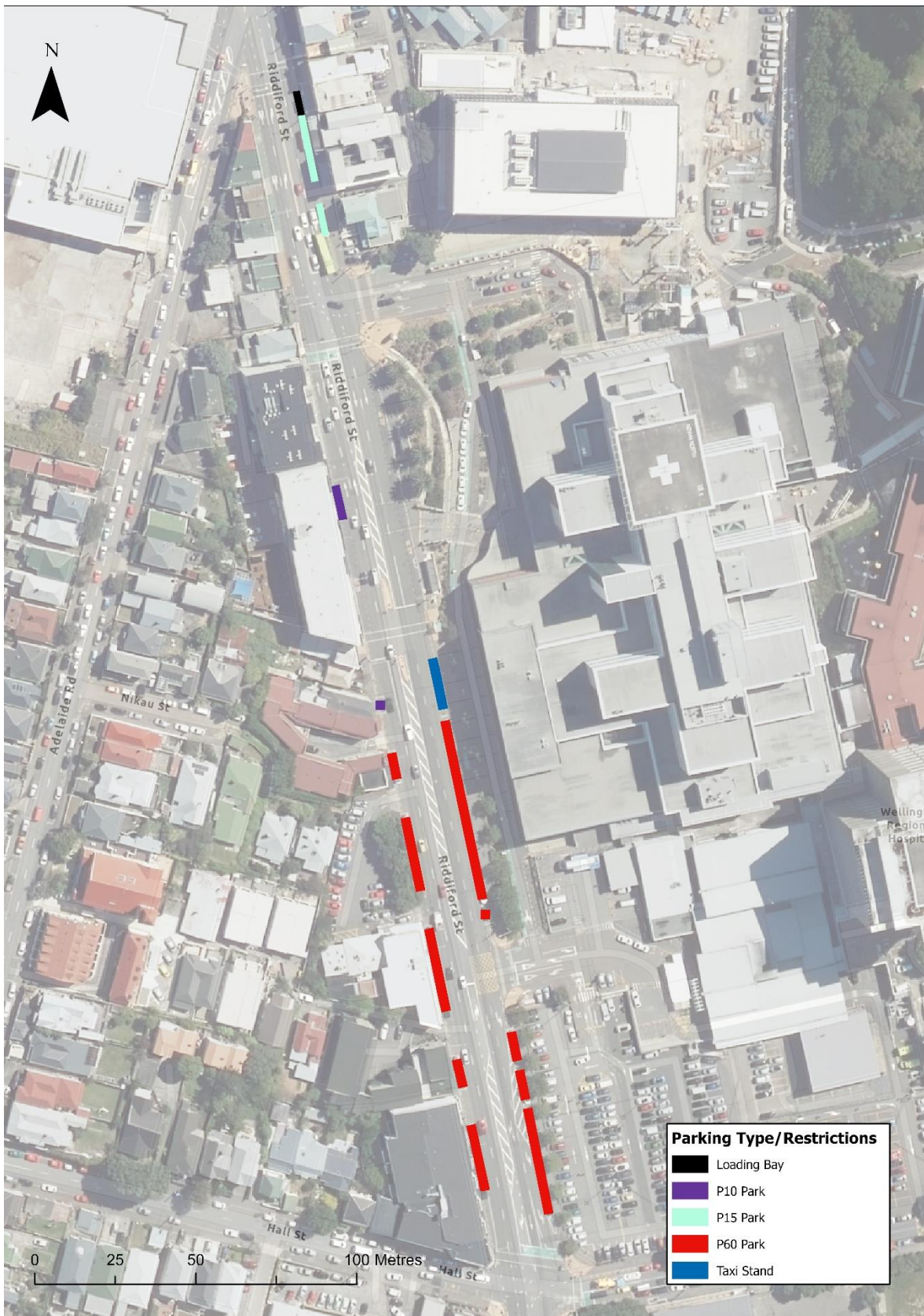
Figure 4.1 Current parking on Riddiford Street – John St to Mein St
