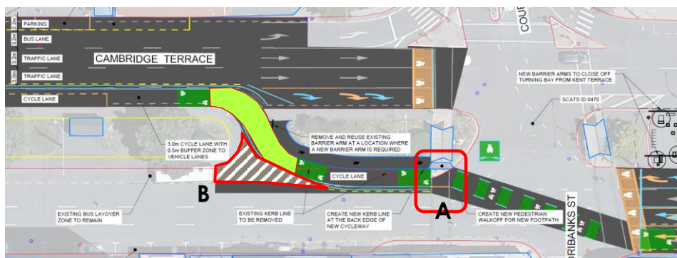
Figure 2-19: Cycle Path transition through Courtenay Place / Majoribanks St intersection to Oriental Parade
