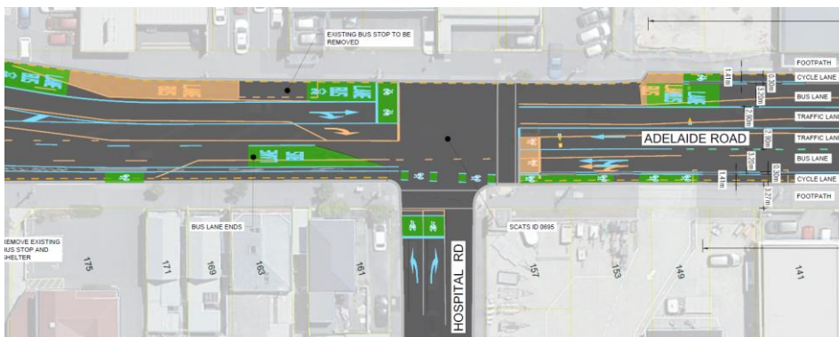
Figure 2-8: Adelaide Road / Hospital Road – southbound lanes shifted right
