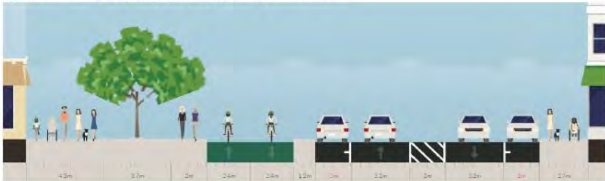
Option 9 - Existing footpaths, two-way cycleway on north side
