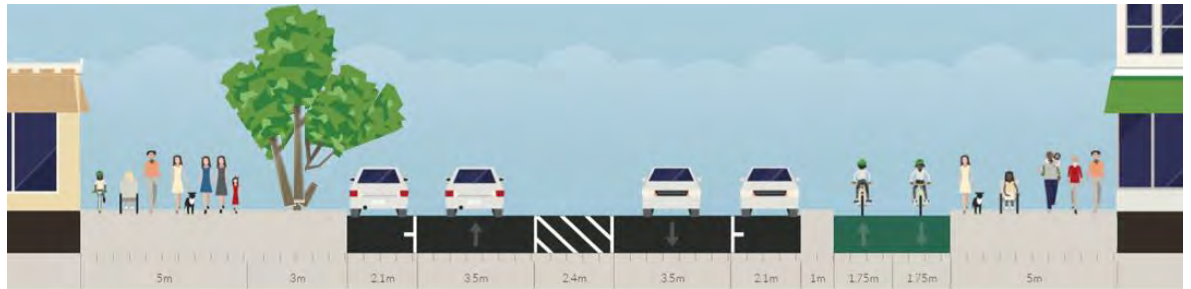
Option 4: 5m footpath on both sides, two-way cycleway on south side.
