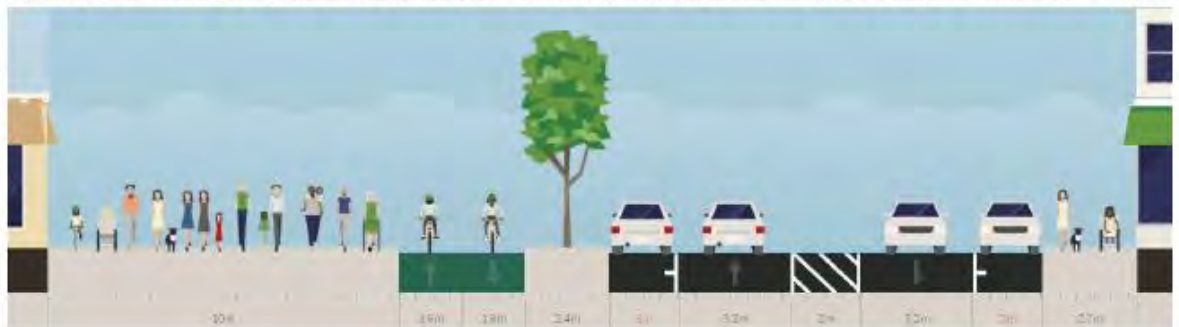
Option 8 - 10m wide footpath on north side, two-way cycle lane on north side, trees on 2.4m wide lane separator
