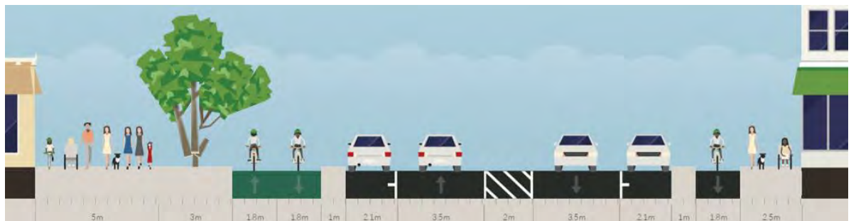
Option 6: Existing footpaths, two-way cycleway on north side and peak-hour bus lanes
