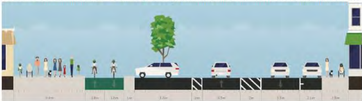
Option 7 - 6.6m wide footpath on north side, two-way cycleway on north side with trees amongst angle parking
