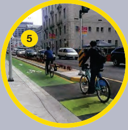
Separated Cycle Lane/Path Contraflow
