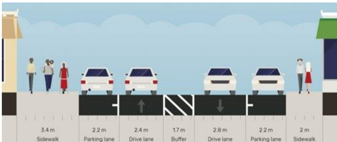
Figure 56: Segment KR-MV-2 Existing Cross Section
