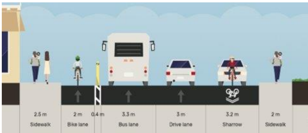
Figure 22: Segment GS-3 Cross Section Including the Selected Bike and Bus Improvement Design
