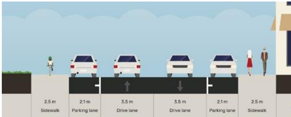
Figure 6: Segment GS-1 Existing Cross Section
