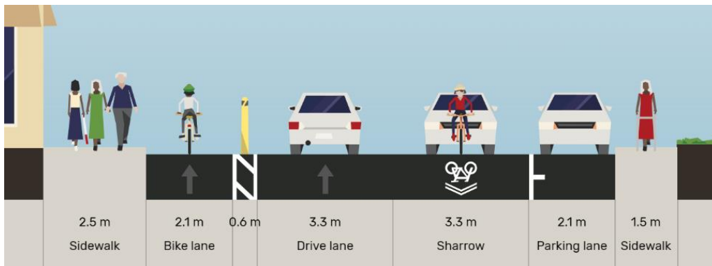
Figure 15: Segment GS-2 Cross Section Including the Selected Bike and Bus Improvements Design
