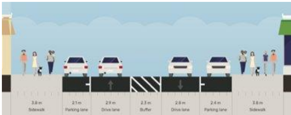
Figure 71: Segment KR-SKR-1 Existing Cross Section
