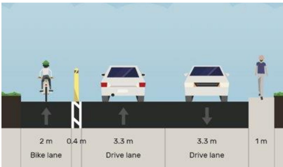
Figure 36: Segment CS-2 Cross Section Including the Selected Bike and Bus Improvement Design
