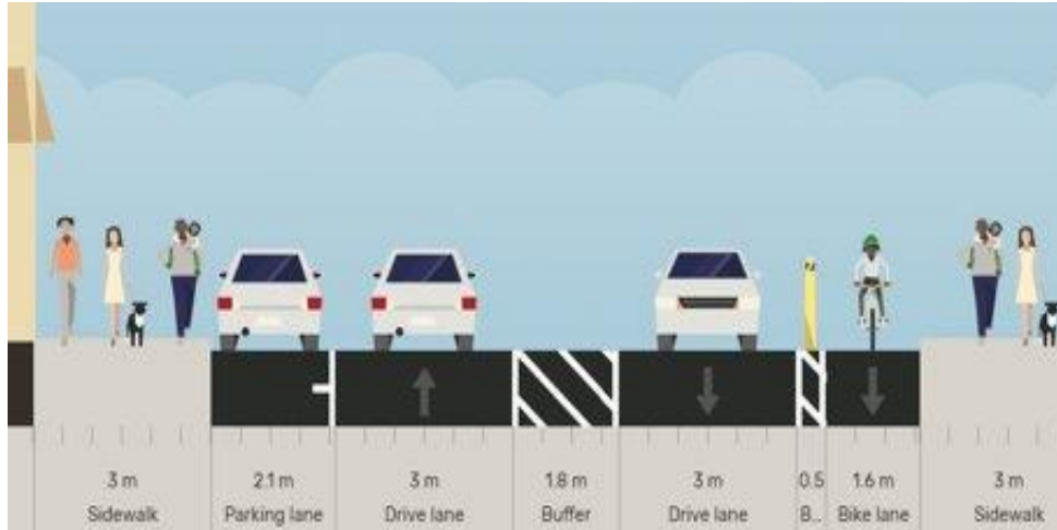
Figure 87: Segment KR-SKR-3 Cross Section Including the Selected Bike and Bus Improvement Design
