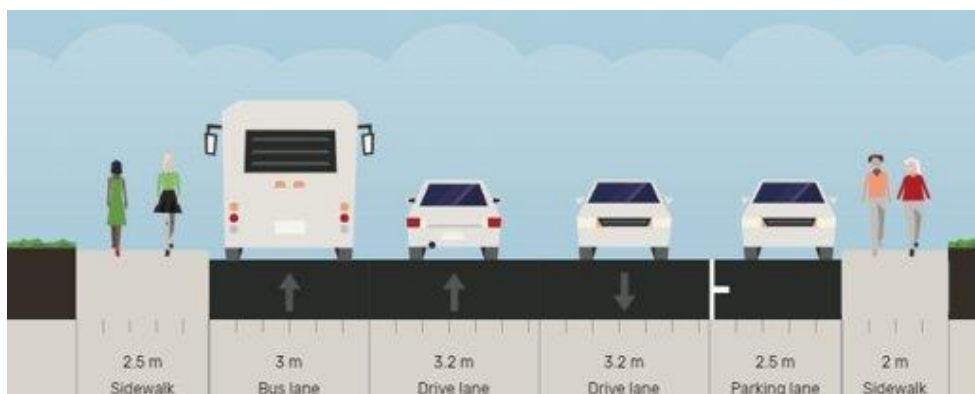
Figure 20: Segment GS-3 Existing Cross Section
