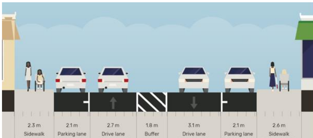
Figure 63: Segment KR-MV-3 Existing Cross Section
