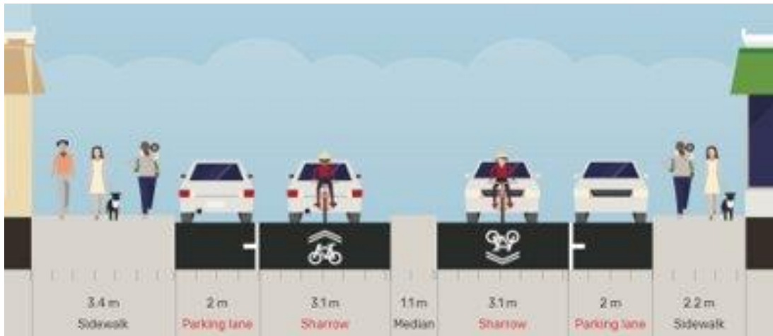
Figure 58: Segment KR-MV-2 Cross Section Including the Selected Bike and Bus Improvement Design
