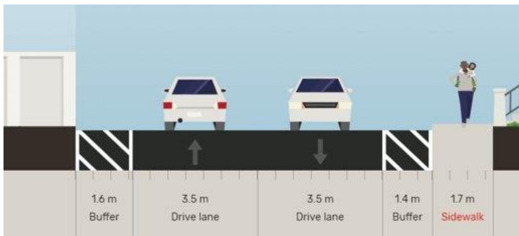
Figure 49: Segment KR-MV-1 Existing Cross Section
