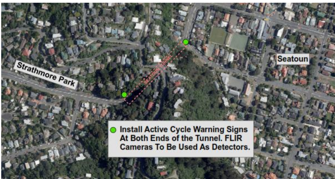
Figure 51 Seatoun Tunnel safety improvements
