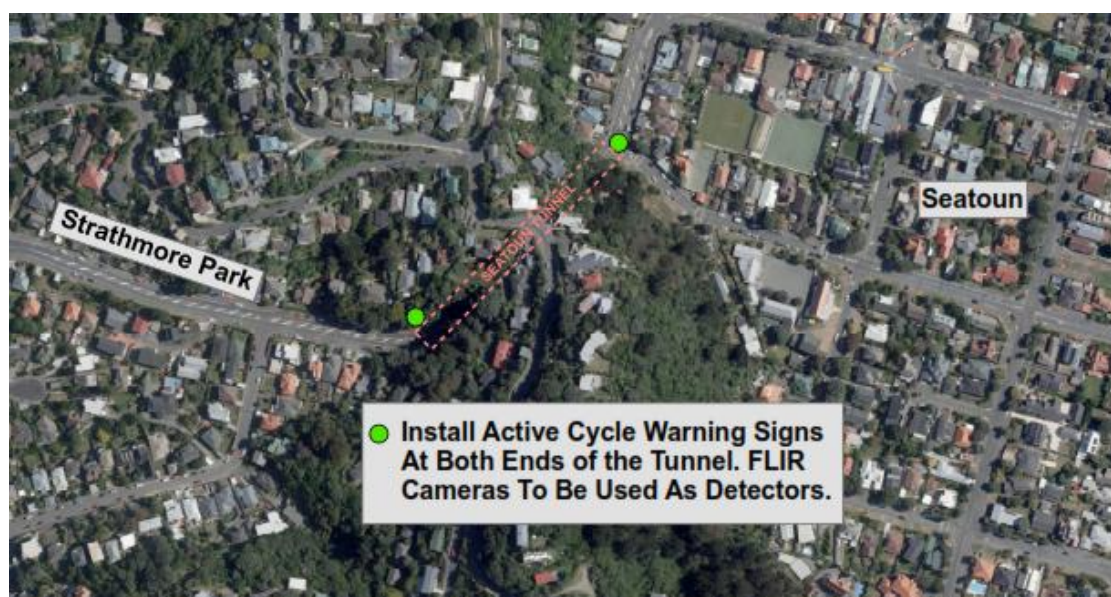
Figure 9 Seatoun Tunnel Safety Improvements
