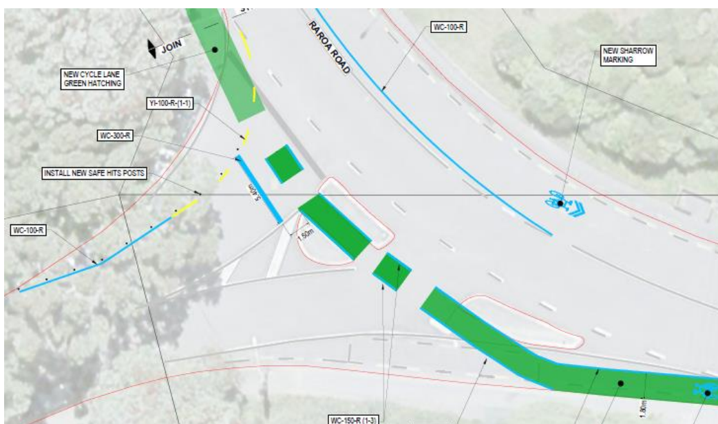
Figure 3.3-1: Holloway Road intersection design
