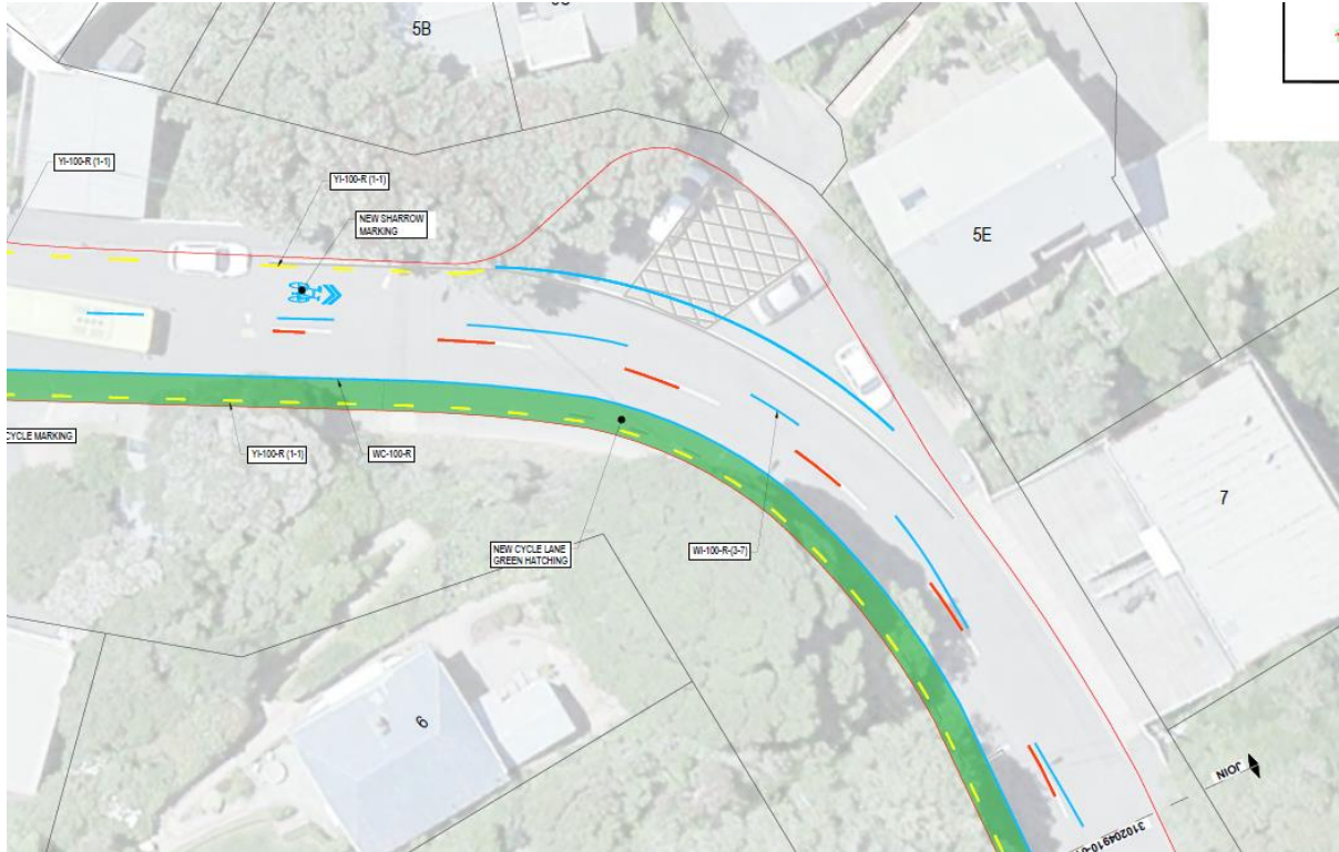
Figure 2.4-1: Cycle lane on inside of curve, Raroa Road
